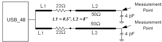
Figure 8. Single-ended USB_48 Clock Double Load Configuration
