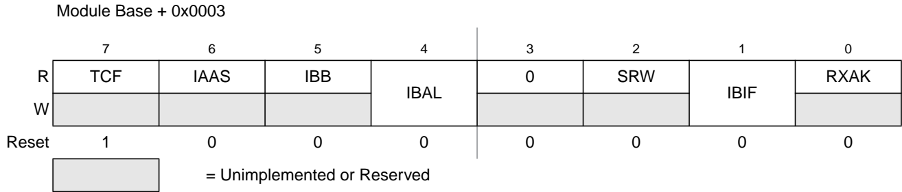
Figure 12-7. IIC Bus Status Register (IBSR)
