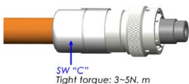
Step 9: Attach and tighten backshell as shown
