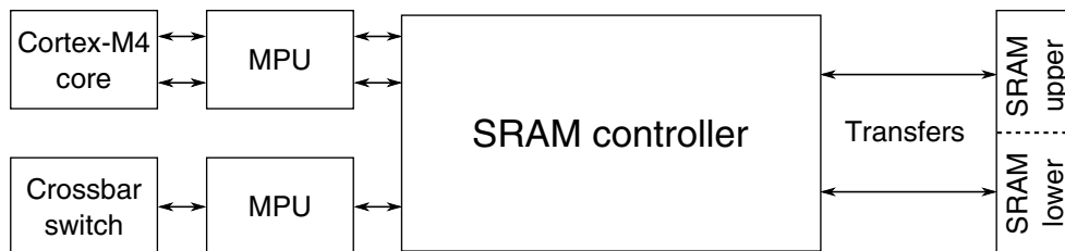
Figure 3-27. SRAM controller configuration
