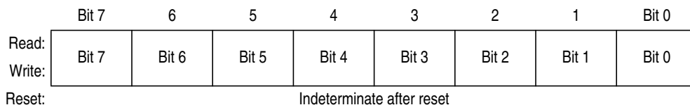
Figure 16-15. TIM1 Channel Register Low (T1CHxL)
