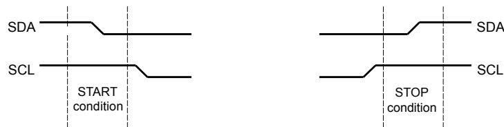
Figure 15-3. START and STOP Conditions
