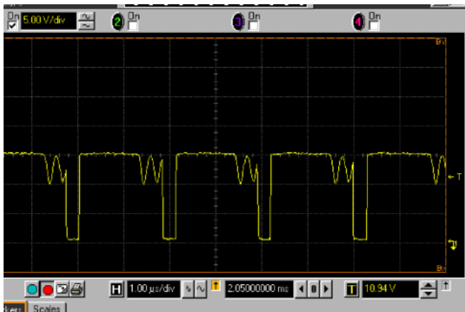
FIGURE 7. BOOST SWITCH NODE AT 100mA (PARTIAL DISCONTINUOUS)
