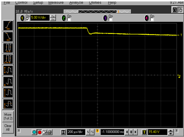
FIGURE 10. VLNB TRANSITIONS FROM 18.3V TO 13.3V
