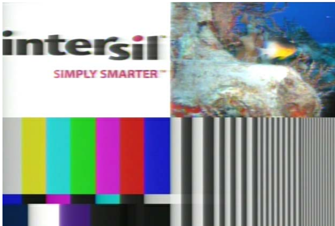
FIGURE 33. TEST PATTERN IMAGE AFTER 4000 FEET OF UNCOMPENSATED RG-59 COAX
