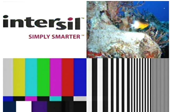
FIGURE 34. TEST PATTERN IMAGE AFTER 4000 FEET OF RG-59 COAX WITH ISL59602 (OR BETTER)
