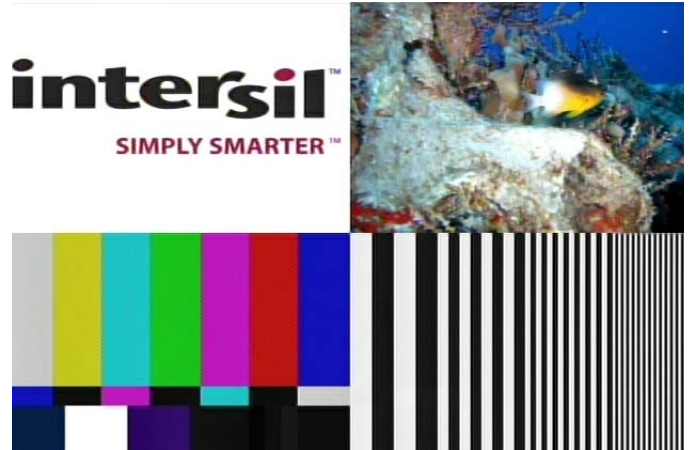
FIGURE 14. TEST PATTERN IMAGE AFTER 4000 FEET OF CAT 5 WITH ISL59604 (OR BETTER)
