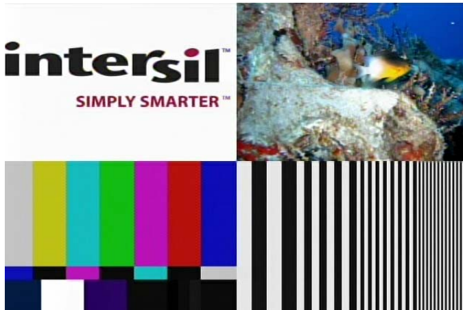
FIGURE 21. TEST PATTERN IMAGE AFTER 1000 FEET OF UNCOMPENSATED RG-59 COAX
