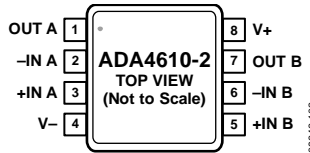
Figure 5. ADA4610-2 Pin Configuration, 8-Lead MSOP (RM Suffix)
