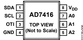
Figure 7. AD7416 Pin Configuration (SOIC/MSOP)
