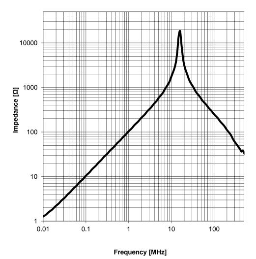
GENERAL TOLERANCE PROJECTION METHOD CREATED CHECKED Würth Elektronik eiSos GmbH & Co. KG **EMC & Inductive Solutions** KaS BMoe DIN ISO 2768-1m Max-Eyth-Str. 1 74638 Waldenburg **WE-MAIA SMD Power Inductor** Tel. +49 (0) 79 42 945 - 0 ORDER CODE www.we-online.com 78438335150 eiSos@we-online.com DATE (YYYY-MM-DD) BUSINESS UNIT REVISION STATUS PAGE 001.004 Valid 3/7 3015 2017-04-17 eiSos **WÜRTH ELEKTRONİK**
