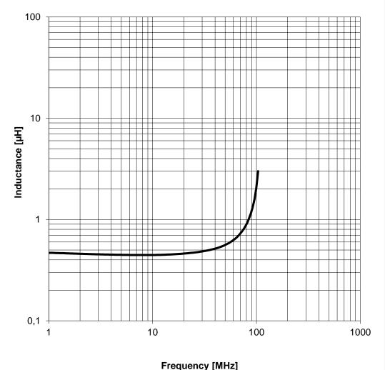
CHECKED GENERAL TOLERANCE CREATED Würth Elektronik eiSos GmbH & Co. KG EMC & Inductive Solutions KaS DDi DIN ISO 2768-1m Max-Eyth-Str. 1 74638 Waldenburg **WE-PMI Power Multilayer Inductor** Tel. +49 (0) 79 42 945 - 0 www.we-online.com 74479887147C eiSos@we-online.com DATE (YYYY-MM-DD) BUSINESS UNIT REVISION STATUS PAGE 001.000 Valid 3/6 2015-11-10 **WÜRTH ELEKTRONİK**
