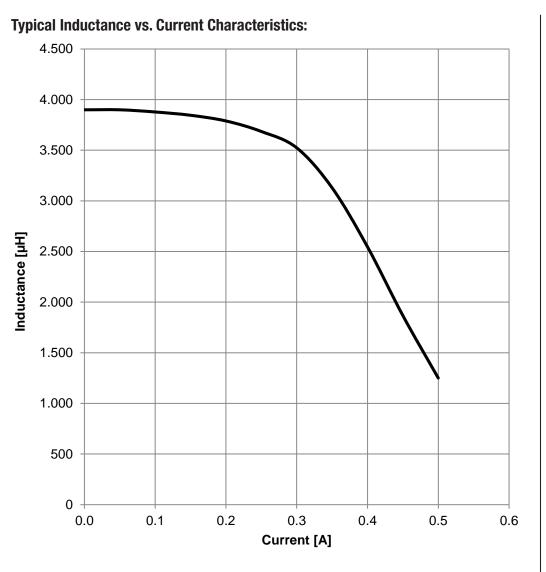
CHECKED GENERAL TOLERANCE PROJECTION METHOD CREATED Würth Elektronik eiSos GmbH & Co. KG KaS StV DIN ISO 2768-1m **WE-TI Radial Leaded Wire Wound** Inductor ORDER CODE 7447720392 DATE (YYYY-MM-DD) BUSINESS UNIT REVISION STATUS PAGE 004.000 Valid 2/6 8095 2016-06-16 eiSos **WÜRTH ELEKTRONİK**
