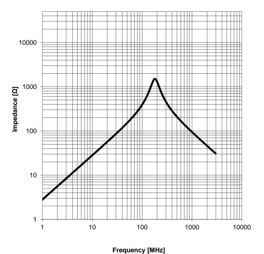
GENERAL TOLERANCE PROJECTION METHOD CREATED CHECKED Würth Elektronik eiSos GmbH & Co. KG EMC & Inductive Solutions KaS DDe DIN ISO 2768-1m Max-Eyth-Str. 1 74638 Waldenburg **WE-MAPI SMD Shielded Power** Tel. +49 (0) 79 42 945 - 0 Inductor ORDER CODE www.we-online.com 744383430047 eiSos@we-online.com DATE (YYYY-MM-DD) BUSINESS UNIT REVISION STATUS PAGE 2010 001.002 Valid 3/7 2018-02-01 eiSos **WÜRTH ELEKTRONİK**
