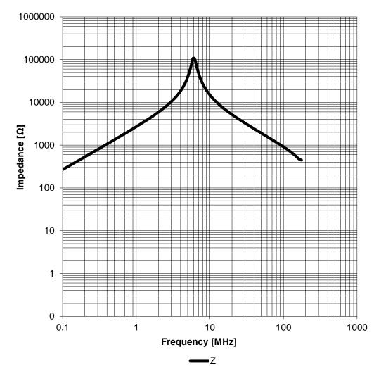
GENERAL TOLERANCE PROJECTION METHOD CREATED CHECKED Würth Elektronik eiSos GmbH & Co. KG JRS **EMC & Inductive Solutions** PaDi DIN ISO 2768-1m Max-Eyth-Str. 1 74638 Waldenburg **WE-TPC SMD Shielded Tiny Power** Tel. +49 (0) 79 42 945 - 0 Inductor ORDER CODE www.we-online.com 744052471 eiSos@we-online.com DATE (YYYY-MM-DD) REVISION BUSINESS UNIT PAGE 2/6 5818 007.005 Valid 2016-12-12 eiSos **WÜRTH ELEKTRONİK**
