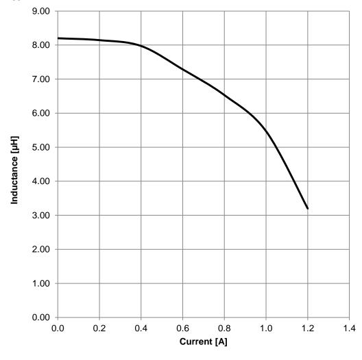
GENERAL TOLERANCE PROJECTION METHOD CREATED CHECKED Würth Elektronik eiSos GmbH & Co. KG JRS **EMC & Inductive Solutions** PaDi DIN ISO 2768-1m Max-Eyth-Str. 1 74638 Waldenburg **WE-TPC SMD Shielded Tiny Power** Tel. +49 (0) 79 42 945 - 0 Inductor ORDER CODE www.we-online.com 744043008 eiSos@we-online.com DATE (YYYY-MM-DD) REVISION STATUS BUSINESS UNIT PAGE Valid 2/6 4828 006.005 2016-12-12 eiSos **WÜRTH ELEKTRONİK**
