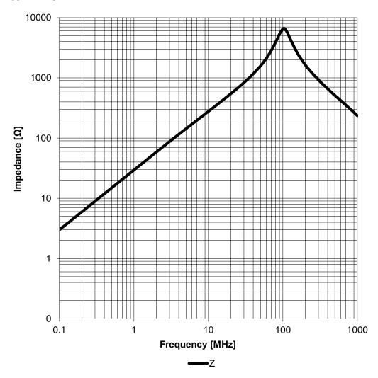
GENERAL TOLERANCE PROJECTION METHOD CREATED CHECKED Würth Elektronik eiSos GmbH & Co. KG EMC & Inductive Solutions JRS PaDi DIN ISO 2768-1m Max-Eyth-Str. 1 74638 Waldenburg **WE-TPC SMD Shielded Tiny Power** Tel. +49 (0) 79 42 945 - 0 Inductor ORDER CODE www.we-online.com 744028004 eiSos@we-online.com DATE (YYYY-MM-DD) BUSINESS UNIT REVISION PAGE 003.005 Valid 2/6 2811 2016-12-05 eiSos **WÜRTH ELEKTRONİK**
