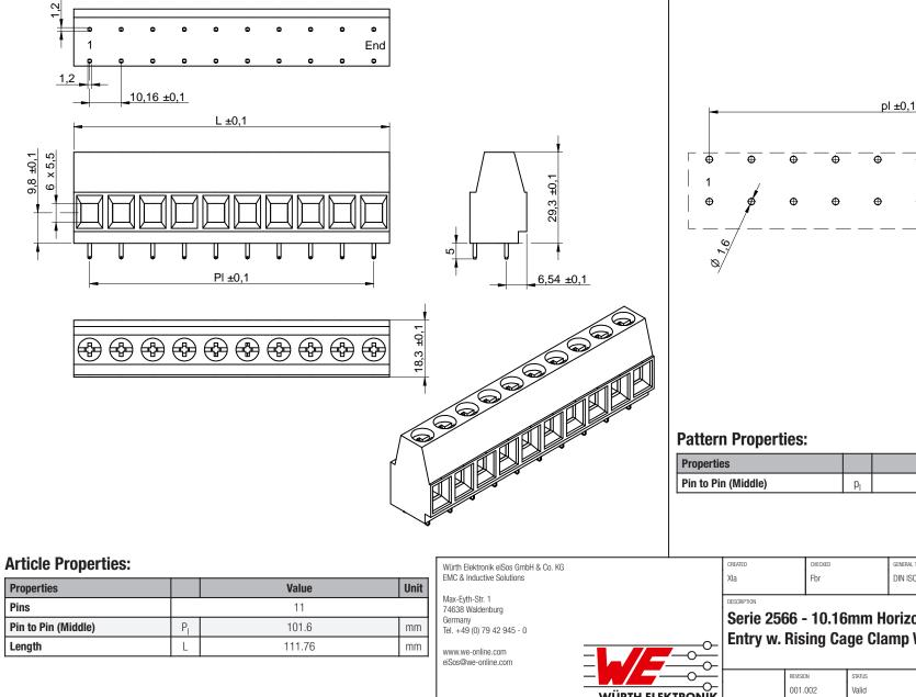
GENERAL TOLERANCE PROJECTION METHOD  $\oplus$ DIN ISO 2768-1m Serie 2566 - 10.16mm Horizontal
