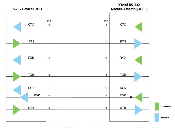
The following diagram shows the DCE Module Assembly (female DB-9 connector) wired to a DCE device (RS-232, male DB-9).
