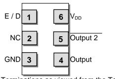
Terminations as viewed from the Top NOTE: XPRESSO LVDS XOs are designed to fit on Industry Standard, 6 pad layouts
