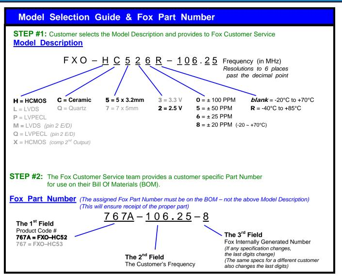
This example, FXO-HC526R-106.25 = HCMOS Output, Ceramic 5 x 3.2mm Package, 2.5V, ±25 PPM Stability, -40 to +85°C Temperature Range, at 106.25 MHz
