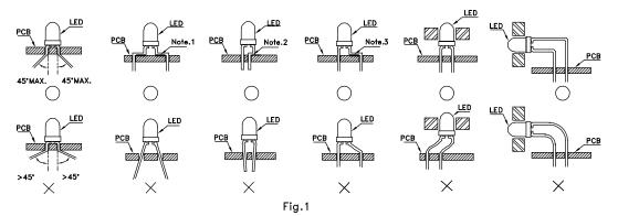
"Correct mounting method "X" Incorrect mounting method
