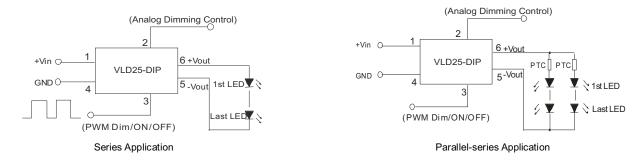
To protect the LED(s), you could connect a PTC to input of all channels as shown in application circuit. Note: Negative output terminal should not conneted to GND. Module may be damaged.
