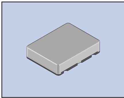
The VC-TXO-39SM is a VC (Voltage Controlled) TCXO (Temperature Compensated Crystal Oscillator) featuring very tight stability over a wide temperature range. The small SMD ceramic package measures 11.4 x 9.6 x 2.3 mm. The voltage control has a tuning range of  $\pm 12$  ppm typical. The low profile package is ideal for wireless communications applications.
