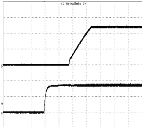
Figure 7: Turn-on transient at zero load current (5 ms/div). V_{in}=48V . Top Trace: V_{out} , 5.0V/div; Bottom Trace: ON/OFF input, 2V/div
