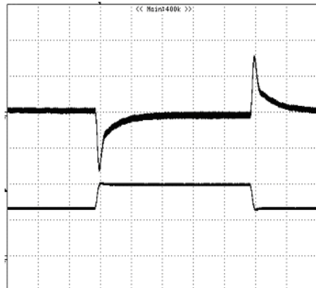
Figure 8: Output voltage response to step-change in load current (75%-50%-75% of I_{o, max} ; di/dt = 0.1A/\mu s ). Load cap: 10 \mu F tantalum capacitor and 1 \mu F ceramic capacitor. Top Trace: V_{out} (100mV/div, 200 \mu s /div), Bottom Trace: I_{out} (2A/div). Scope measurement should be made using a BNC cable (length shorter than 20 inches). Position the load between 51 mm to 76 mm (2 inches to 3 inches) from the module
