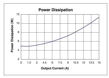
Figure 4 — Power dissipation vs. output current.
