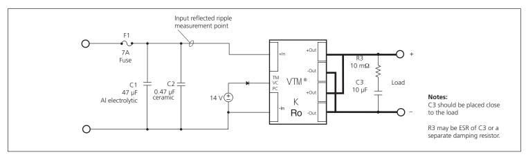
Figure 15 — VTM module test circuit
