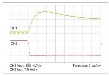
**Figure 8** — 15-0 A load step with 100 μF input capacitance and no output capacitance.
