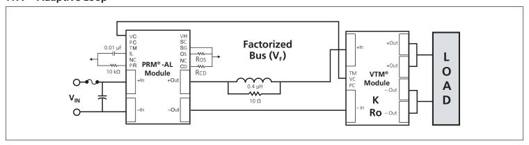
**Figure 18** — The PRM regulator controls the factorized bus voltage,  $V_F$ , in proportion to output current to compensate for the output resistance, Ro, of the VTM current multipler. The VTM module output voltage is typically within 1% of the desired load voltage  $(V_F)$  over all line and load conditions.
