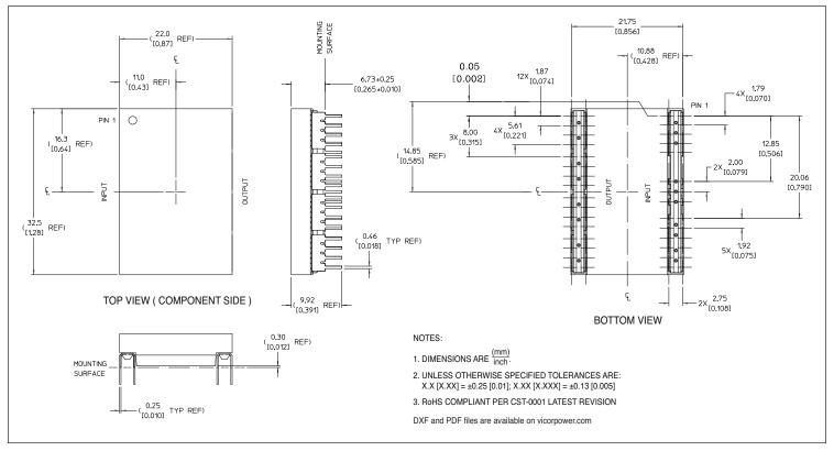
Figure 12 —VTM through-hole module mechanical outline
