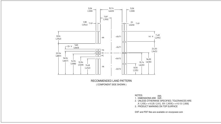
Figure 11 — VTM module J-Lead PCB land layout information; Onboard mounting
