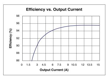
Figure 3 — Efficiency vs. output current.
