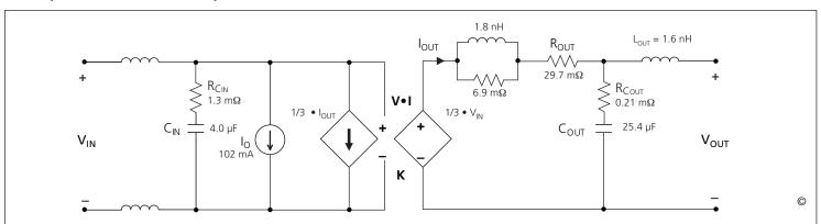
**Figure 17** — This model characterizes the AC operation of the VI Chip VTM including response to output load or input voltage transients or steady state modulations. The model enables estimates or simulations of input and output voltages under transient conditions, including response to a stepped load with or without external filtering elements.
