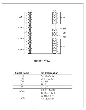
**Figure 9** — VTM current multiplier pin configuration
