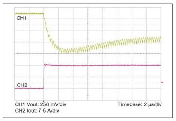
**Figure 7** — 0-15 A load step with 100  $\mu$ F input capacitance and no output capacitance.
