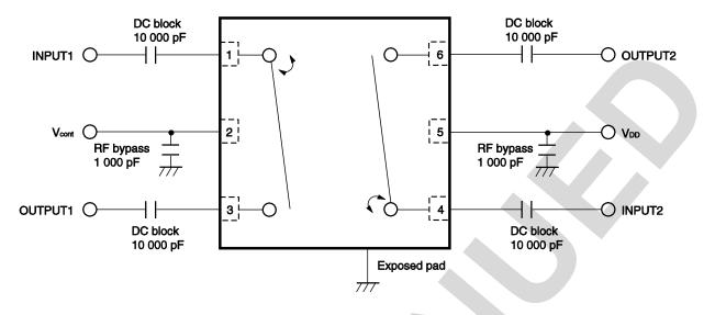
Caution This IC has pull down resistances inside between each RF line and GND line, which bias each RF pin internally to GND, then the IC cannot be used for DC switching.
