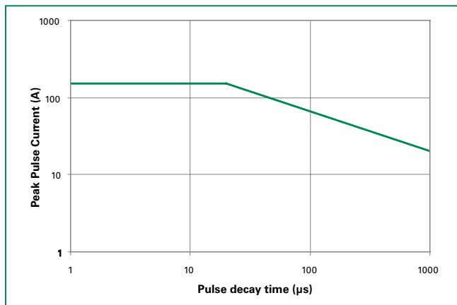
Figure 1: Non-repetitive Peak Pulse Current vs. Pulse Time
