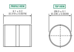
'R' Type Radial Lead Devices (SL1003AxxxR and SL1003AxxxRF)
