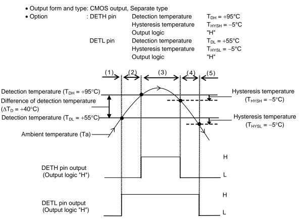
Figure 11 Timing Chart for CMOS Output and Separate Type
