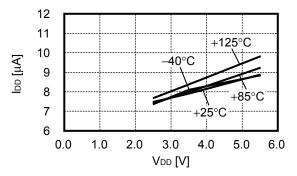
2. Output current "H" of DETH / DETL pin vs. Power supply voltage characteristics (CMOS output product only)
