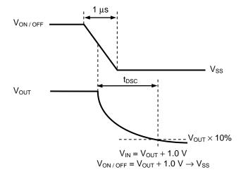
Figure 34 Measurement Condition of Discharge Time
