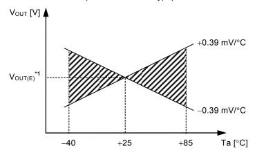
\*1.  $V_{OUT(E)}$  is the value of the output voltage measured at Ta =  $+25^{\circ}$ C.
