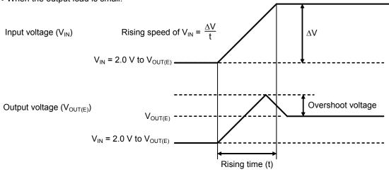
Figure 14 V<sub>IN</sub> and Overshoot Voltage
