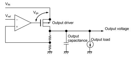
Figure 13 Circuit Diagram
