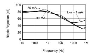
S-1112B30 (Ta = 25°C)  $V_{\text{IN}} = 4.0 \text{ V, } C_{\text{OUT}} = 0.47 \text{ } \mu\text{F}$
