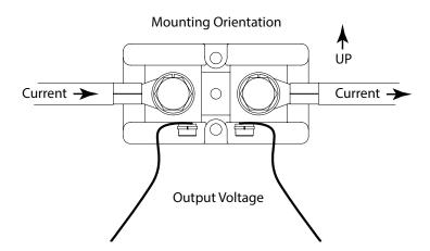
**Operating Current Derating:** For continuous operation, it is recommended that shunts are not run at more than two thirds (2/3) the rated current under normal conditions per IEEE standards for DC instrument shunts. At ambient temperatures above 40°C, the current must be further derated to prevent damage.
