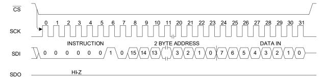
The Adesto RM25C family is capable of a 64-byte write operation.
