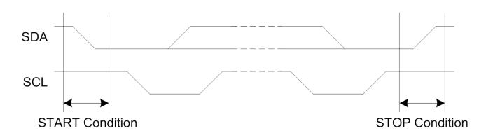
Every byte put on the SDA line must be 8 bits long. The number of bytes that can be transmitted per transfer is unrestricted. Each byte must be followed by an acknowledge bit; therefore, the number of clock cycles to transfer one byte is nine. Data is transferred with the most significant bit (MSB) first.
