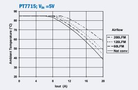
**Note A:** All characteristic data in the above graphs has been developed from actual products tested at 25°C. This data is considered typical for the ISR. **Note B:** SOA curves represent operating conditions at which internal components are at or below manufacturer's maximum rated operating temperatures.
