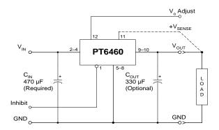
$C_{in}$  = Required 470  $\mu$ F  $C_{out}$  = Optional 330  $\mu$ F
