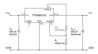
The values of  $(R_1)$  [adjust down], and  $R_2$  [adjust up], can be calculated using the following formulas. Refer to Figure 3-1 for the placement of the required resistor; either  $(R_1)$  or  $R_2$ , as appropriate.
