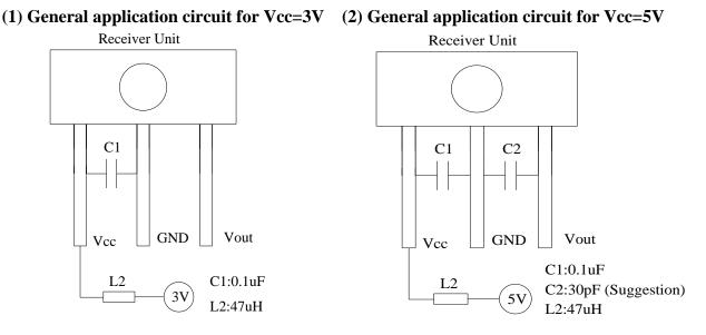
Note: For having good coupling, the C1,C2 capacitor must be placed within 7mm
