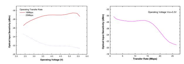
**Note:** Before using the PLR135 device, please confirm the minimum sensitivity at different operating voltage and transmission rate.
