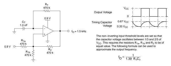
Figure 34. 0.9 V Square Wave Oscillator
