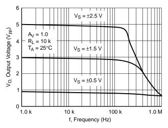
Figure 8. Output Voltage vs. Frequency
