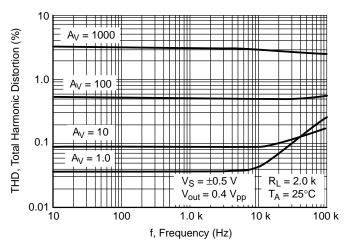
$A_V = 1000$ THD, Total Harmonic Distortion (%) 10 CT 1 1.0  $A_V = 100$  $A_{V} = 10$  $A_V = 1.0$  $V_S = \pm 0.5 V$  $T_A = 25^{\circ}C$  $V_{out} = 0.4 V_{pp}$ 0.01 10 100 1.0 k 10 k 100 k f, Frequency (Hz)
