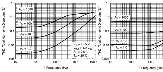
Figure 16. Total Harmonic Distortion vs. Frequency with 5.0 V Supply
