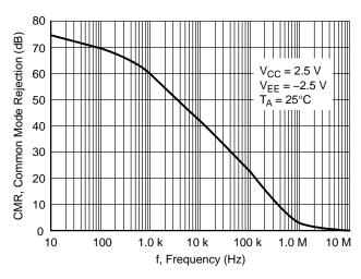
Figure 9. Common Mode Rejection vs. Frequency
