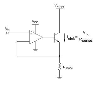
Figure 38. High Compliance Current Sink
