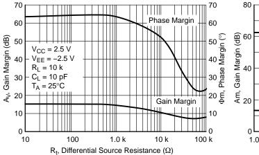
Figure 22. Gain and Phase Margin vs. Differential Source Resistance
