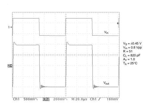
Figure 33. Small Signal Transient Response with Large Capacitive Load and Isolation Resistor.
