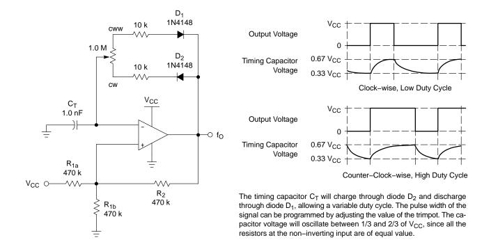
Figure 35. Variable Duty Cycle Pulse Generator
