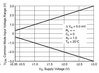
Figure 29. Common-Mode Input Voltage Range vs. Power Supply Voltage
