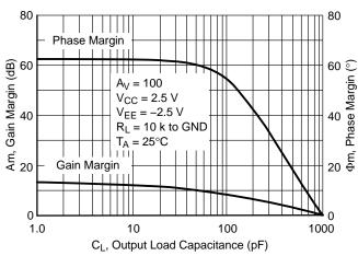
Figure 23. Gain and Phase Margin vs.
