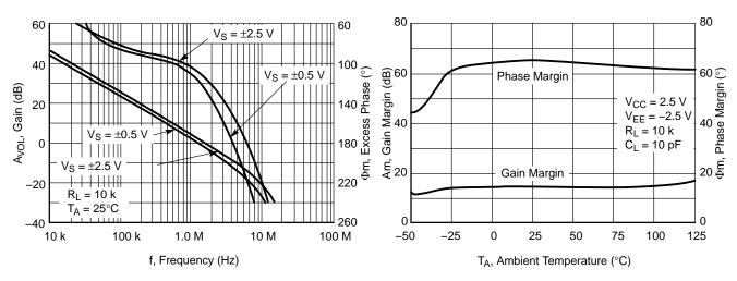
Figure 20. Voltage Gain and Phase vs. Frequency
