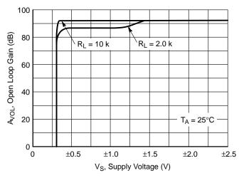
Figure 26. Open Loop Voltage Gain vs. Supply Voltage
