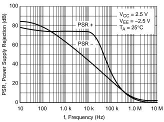
Figure 10. Power Supply Rejection vs. Frequency
