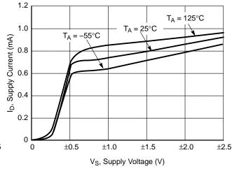
Figure 13. Supply Current vs. Supply Voltage
