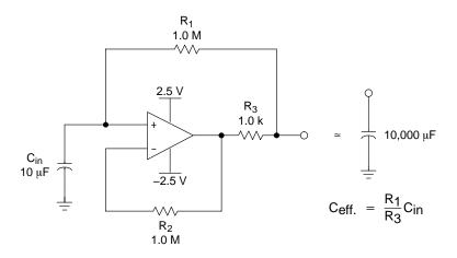
Figure 36. Positive Capacitance Multiplier
