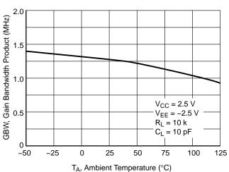
Figure 19. Gain Bandwidth Product vs. **Temperature**
