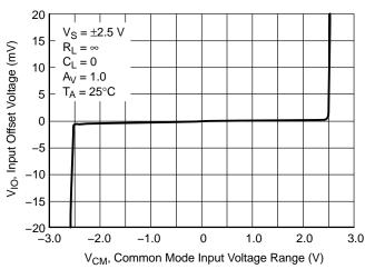
Figure 27. Input Offset Voltage vs. Common Mode Input Voltage Range  $V_S = \pm 2.5 \text{ V}$
