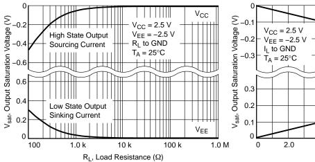
Figure 2. Split Supply Output Saturation vs. Load Resistance
