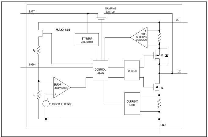
Figure 2. MAX1724 Simplified Functional Diagram
