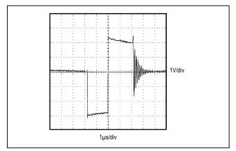
Figure 5. LX Ringing Without Damping Switch (MAX1723)
