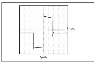
Figure 6. LX Ringing With Damping Switch (MAX1722/MAX1724)
