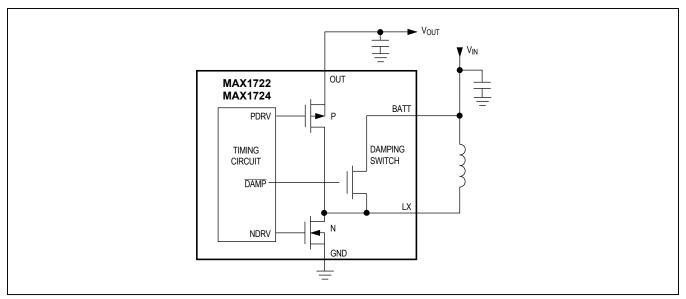
Figure 4. Simplified Diagram of Damping Switch
