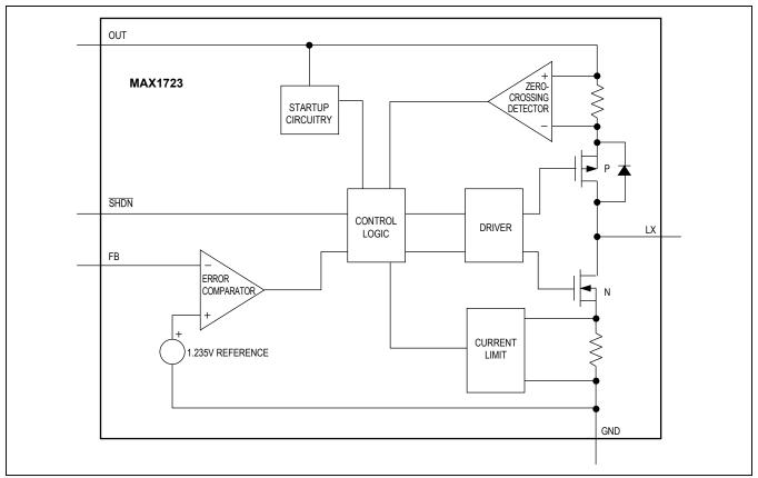
Figure 1. MAX1723 Simplified Functional Diagram
