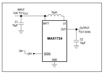
Figure 8. MAX1724 Standard Application Circuit
