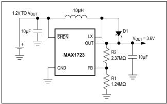
Figure 3. MAX1723 Single-Cell Operation
