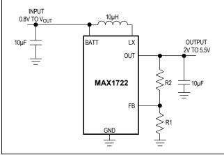
Figure 7. Adjustable Output Circuit
