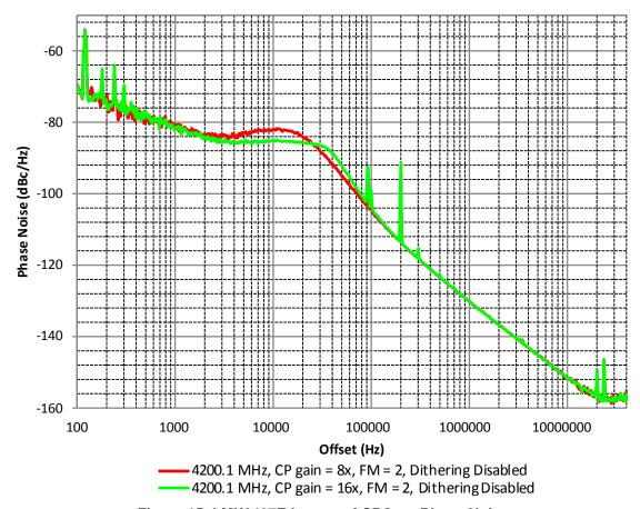
Figure 15. LMX2487E Impact of CPG on Phase Noise
