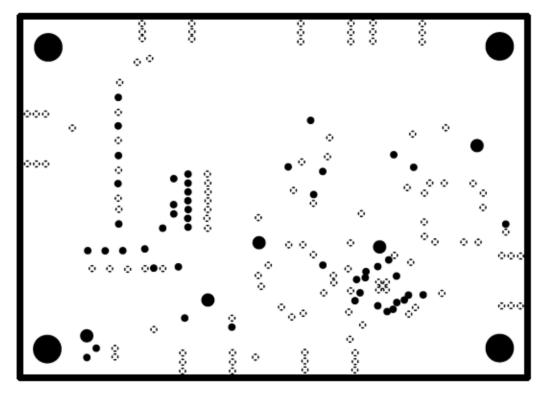
Figure 9. Layer #2 - RF Ground Plane
