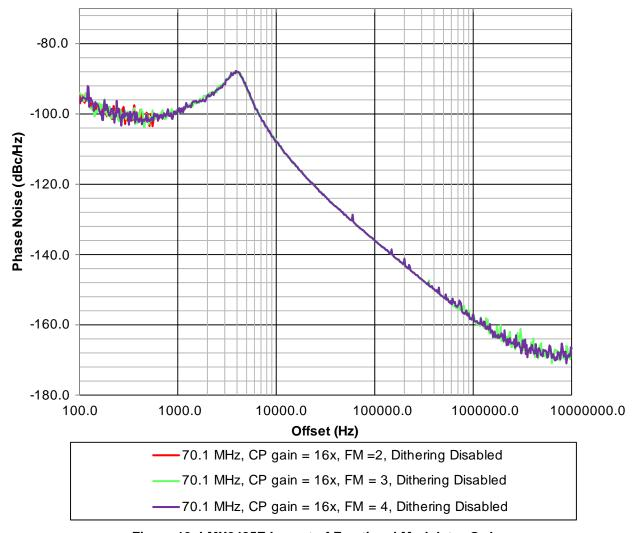
Figure 13. LMX2485E Impact of Fractional Modulator Order
