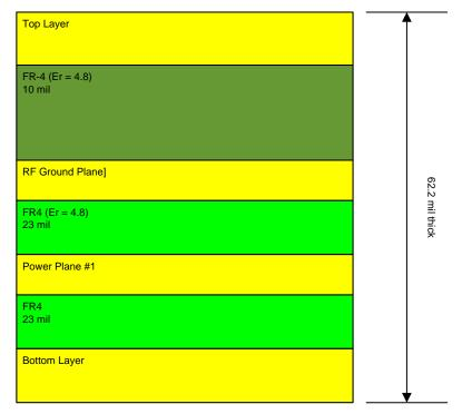
Figure 7. PCB Layers
