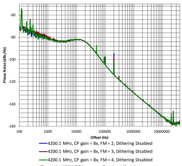
Figure 16. LMX2487E Impact on Fractional Modulator
