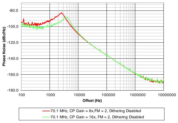
Figure 12. Impact of CPG on Phase Noise
