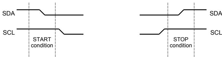
Figure 16-3. START and STOP Conditions
