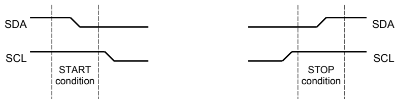
Figure 14-3. START and STOP Conditions
