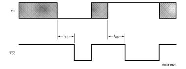
FIGURE 1. LM3712 Reset Time with  $\overline{\text{MR}}$
