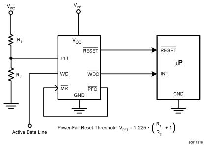
FIGURE 3. Monitoring Two Critical Supplies Plus Dataline
