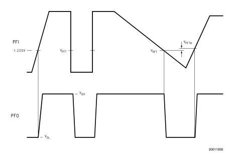
FIGURE 2. PFI Comparator Timing Diagram
