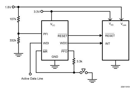
FIGURE 4. Monitoring Two Supplies plus Manual Reset And Dataline
