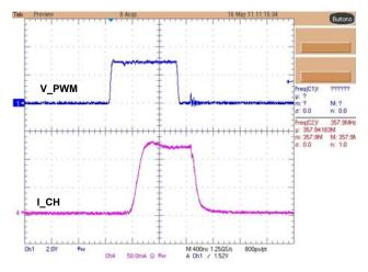
FIGURE 19. MINIMUM DIMMING DUTY CYCLE (0.05%,  $\rm f_{DIM}$ : 500Hz,  $\rm I_{CH}$  = 120mA, DIRECT PWM MODE)
