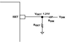
FIGURE 21. LED CURRENT CONTROL WITH VDIM
