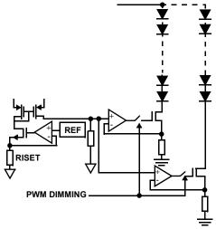
FIGURE 20. SIMPLIFIED CURRENT SOURCE CIRCUIT
