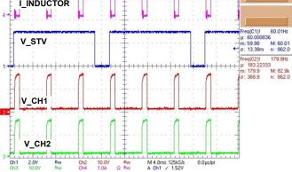
FIGURE 16. V<sub>SYNC</sub> ENABLED DIMMING WITHOUT PHASE SHIFT (V<sub>IN</sub>: 19V, I<sub>CH</sub>: 120mA, LEDs: 4P18S, 180Hz OUTPUT PHASE AND FREQUENCY LOCKED TO 60Hz STV)
