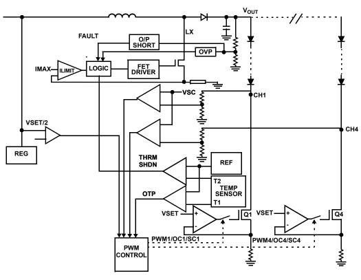
FIGURE 26. SIMPLIFIED FAULT PROTECTIONS
