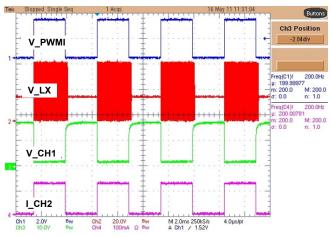
FIGURE 11. DIRECT PWM DIMMING (V<sub>IN</sub>: 19V, LEDs: 4P18S,  $f_{DIM}$ : 200Hz)
