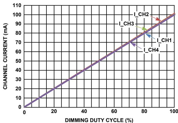
FIGURE 2. PWM DIMMING LINEARITY
