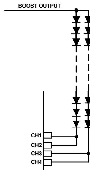
FIGURE 27. GROUPING MULTIPLE CHANNELS FOR HIGH CURRENT APPLICATIONS
