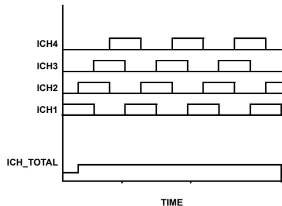
FIGURE 24. PHASE SHIFT PWM DIMMING AT 50% DUTY CYCLE
