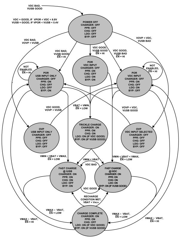
FIGURE 4. STATE DIAGRAM FOR CHARGER FUNCTIONS
